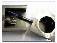
Remove the firepot assembly by sliding it away from the auger box
