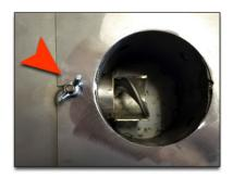
Remove the wingnut that is securing the firepot to the auger box
